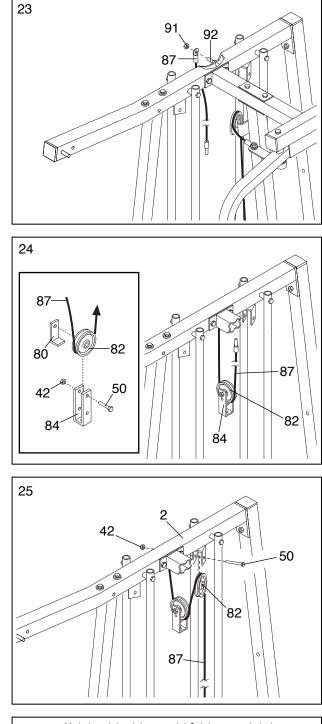
24. See the inset drawing. Attach a 3 1/2" Pulley (82) and a Cable Trap (80) to the upper hole in a Large "U" Bracket (84) with a 3/8" x 2" Bolt (50) and a 3/8" Nylon Locknut (42). Make sure the Cable Trap is inside the Large "U" Bracket. Note: This may come pre-assembled.
